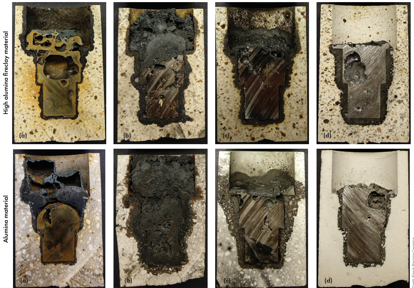
Figure 1. Corrosion testing of high alumina fireclay and alumina crucibles containing (a) cast iron, (b) 304 stainless steel, (c) 400 nickel, and (d) 6061 aluminum.
