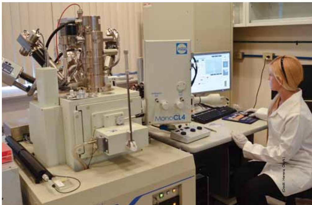
Graduate student Luz Zavala studies cathodoluminescence of doped hydroxyapatite materials to determine dopant distribution in powders and films at CNyN. This laboratory is under the direction of Manuel Herrera.
