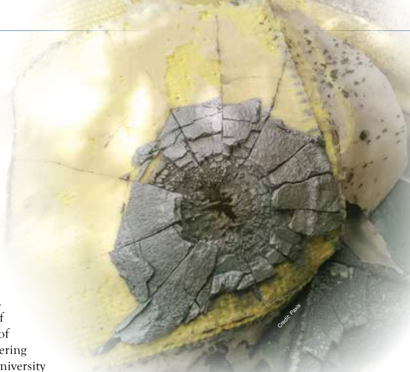
Figure 1. A BorLite reaction-bonded boron carbide armor plate, manufactured by Paxis Ltd. (Savion, Israel), after impact with 7.62X63 AP M2 projectiles. (Image from ACerS Bulletin , August 2017)
