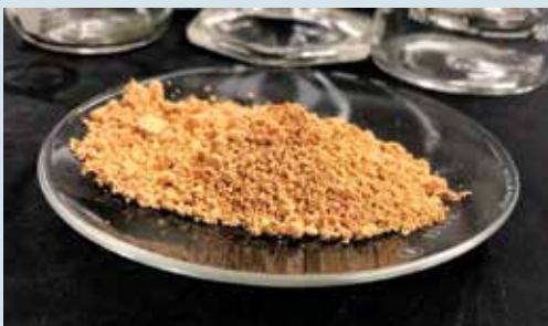
WVU's Rare Earth Extraction Facility produces highly concentrated rare earth products from coal mine drainage. This sample is 87 percent rare earth oxide. Credit: WVU Photo/Chris Vass
