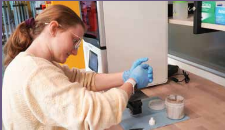
Figure 2. Jane Heffernan prepares a sample as part of her research studying ways to 3D print silicon carbide.
