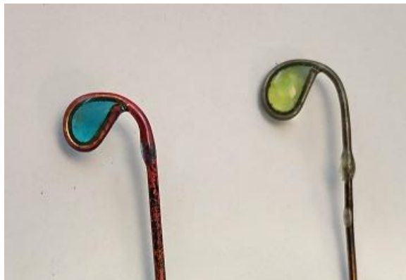
Figure 4. Borax beads formed with copper wire (blue bead) and nichrome wire (green bead)
