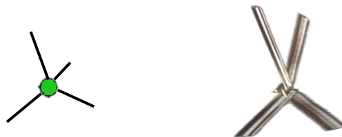
Figure 8: Schematic (left) and model made of zip ties (right) showing the tetrahedral structure.
